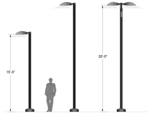
Figure 8 - Commercial Area Light Fixture
